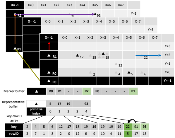
Fig. 6: Lookup of key 22 when the key set is spread across multiple planes. The example shows the worst case where five rays are required to perform the lookup.
